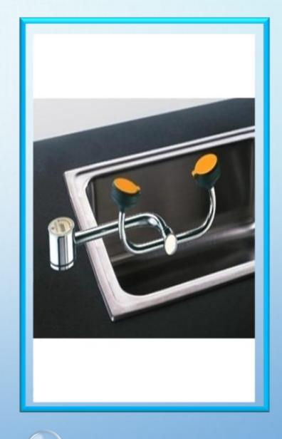
APPLICATION: AUTOFLOW EYE/FACE WASH FOR MOUNTING ON COUNTER NEXT TO SINK. SWINGING THE SPRAY HEAD ASSEMBLY 90 DEGREES HORIZONTALLY OUT OVER SINK ACTIVATES THE WATER FLOW. THE UNIT REMAINS IN OPERATION UNTIL THE SPRAY HEAD ASSEMBLY IS SWUNG BACK INTO THE STORAGE POSITION, CLOSING THE VALVE.
