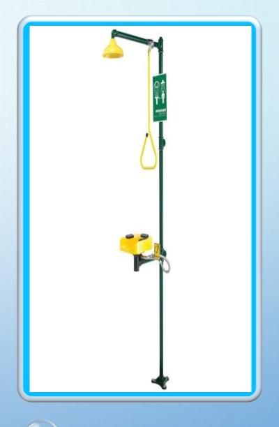
COMBINATION STATION WITH SE-695 EYE/FACE WASH WITH DUAL SPRAY OUTLETS, FLIP TOP DUST COVERS AND YELLOW PLASTIC BOWL. PAINTED GALVANIZED STEEL STANCHION WITH A DELUGE SHOWERHEAD. ACTIVATED BY A HIGH VISIBILITY YELLOW PULL ROD.
