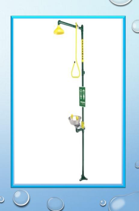
COMBINATION SHOWER WITH SE-690 EYE/FACE WASH WITH DUAL SPRAY OUTLETS, FLIP TOP DUST COVERS AND STAINLESS STEEL BOWL. PAINTED GALVANIZED STEEL STANCHION WITH AN IMPELLER ACTION DELUGE SHOWERHEAD ACTIVATED BY A HIGH VISIBILITY YELLOW PULL ROD.
